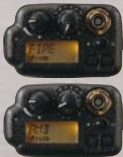
**INVERT ALPHA-DISPLAY** Any one of the programmable PF keys or toggle switch can be set to invert the channel alpha-tags for ease of viewing when the unit is worn on a belt, inside a protective suit or on a chest-pack.
