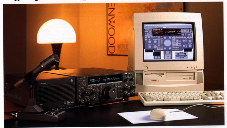
The TS-870S is fully computer-controllable through a built-in 57.6 Kbps interface and Microsoft® Windows™ compatible software (supplied). You can expand the functionality of the rig by setting up virtually any combination of settings (including on/off control) for frequencies, bands, modes, and any other parameters with this software program.
